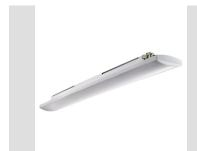
Luminaire with MID power LED (double or single die) equipped with steel sheet heat sink / reflector pre painted in white colour. Body in PC grey RAL7035. Diffuser in PC U.V. ray stabilized. Sealing deposited by automatic machine. Fixing system for wall, ceiling or suspension with harmonic steel springs, and wide adjustable fixing range. Quick connector integrated in the fixture for wires with12.5mm max. diameter. Electronic LED driver with power factor correction.
